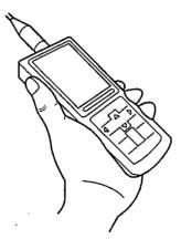
**⑤Clean the cell** ..... Clean amply the electric conductivity cell and the immersed part such as the cable with pure water and wipe off the water drops with tissue paper, etc.
