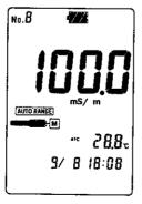
Measurement screen of electric conductivity mode
