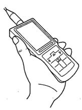
Stop the sample flow ..... After reading the measured value, stop the sample water flow.
